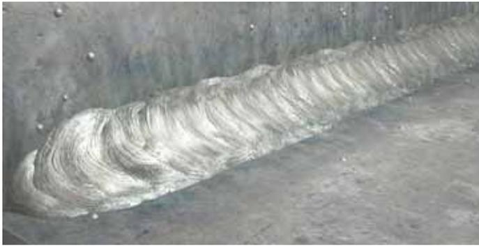
▲ **FIGURE 2** After welding, the student can view the “virtual” finished weldment.
