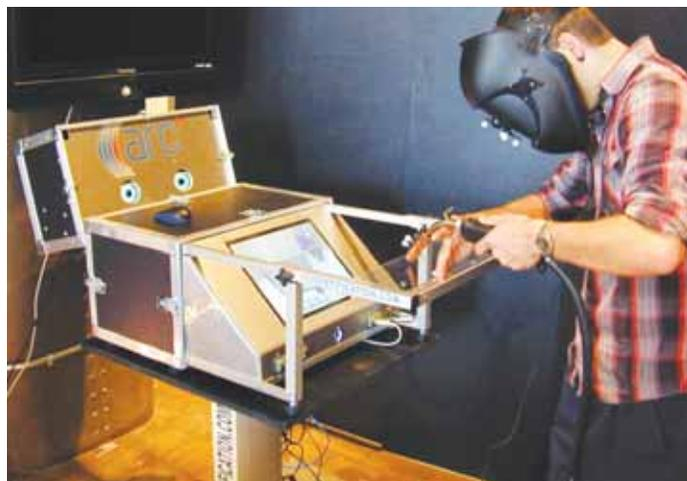
▲ **FIGURE 1** A welder uses the arc+® simulator from 123Certification.
