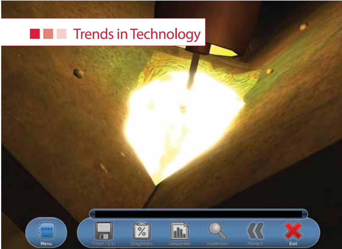
◀ A virtual reality simulation of gas metal arc welding a fillet weld. Source: 123Certification Inc.
