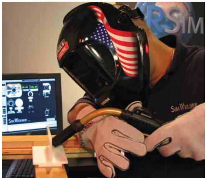
▲ **FIGURE 4** VRSim’s SimWelder™ uses both a virtual graphic display, inside the helmet and strapped to the headband, with a real-world plastic mockup of the weld joint.
