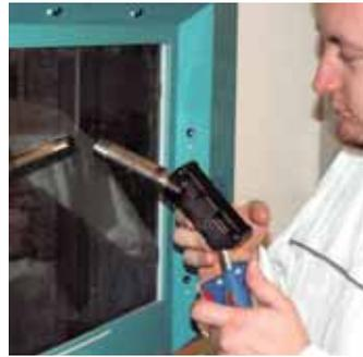
▲ **FIGURE 3** A technician demonstrates the CS WAVE system, which simulates the resulting weld on a screen.
