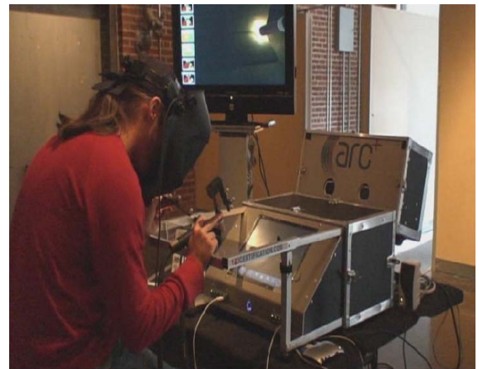
Figure 4: ARC+ welding simulator in action with the GTAW (TIG Welding) for a welder training. Source: 123Certification Inc.
