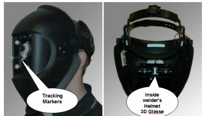
Figure 1: Real Welder Helmet with motion tracking technology Source: 123Certification Inc.
