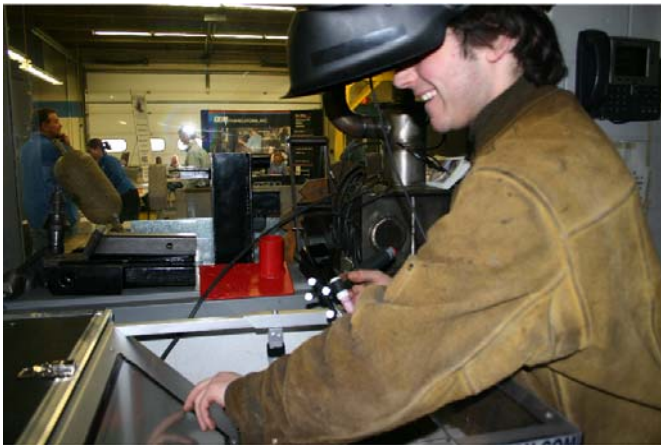
Figure 11: Tactile Screen is used to access the diagnostic allowing the welder to take immediate corrective action, and continuously improve his skills in a safe and enjoyable setting. Source: Chippewa Valley Technical College in Eau Claire, Wisconsin.
