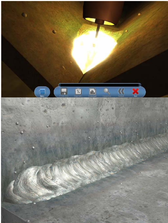
Figure 2: A virtual reality simulation of gas metal arc welding a fillet weld (GTAW). Source: 123 Certification Inc.
