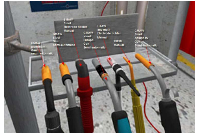
Figure 3: ARC+ simulates all these manual and semi-automatic welding processes Source: 123Certification Inc.
