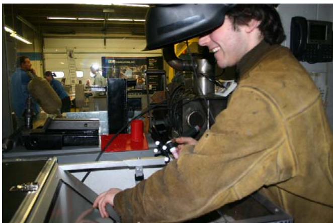
Figure 11: Tactile Screen is used to access the diagnostic allowing the welder to take immediate corrective action, and continuously improve his skills in a safe and enjoyable
