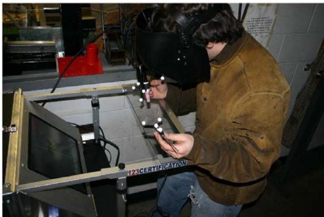
Figure 10: Virtual reality training of gas tungsten arc welding (GTAW). Source: Chippewa Valley Technical College in Eau Claire, Wisconsin.
