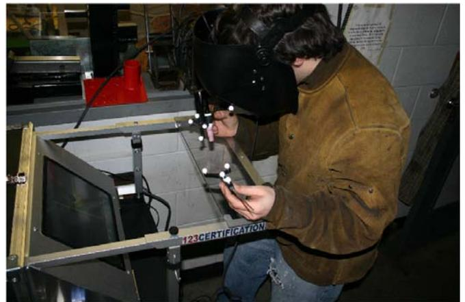
Figure 10: Virtual reality training of gas tungsten arc welding (GTAW).
