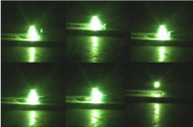
Figure 12: High Speed Pictures of GTAW deposition
