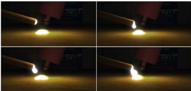
Figure 13: High Speed Images of Virtual GTAW deposition.
